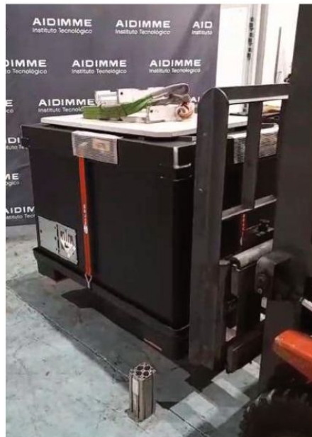
Photograph 2 - Bottom lift test in process
