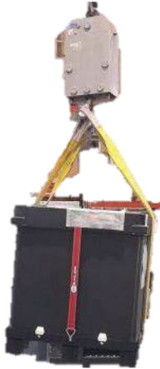
Photograph 4 – Drop test in process.
