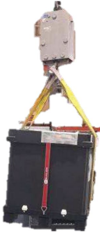
Photograph 4 – Drop test in process.
