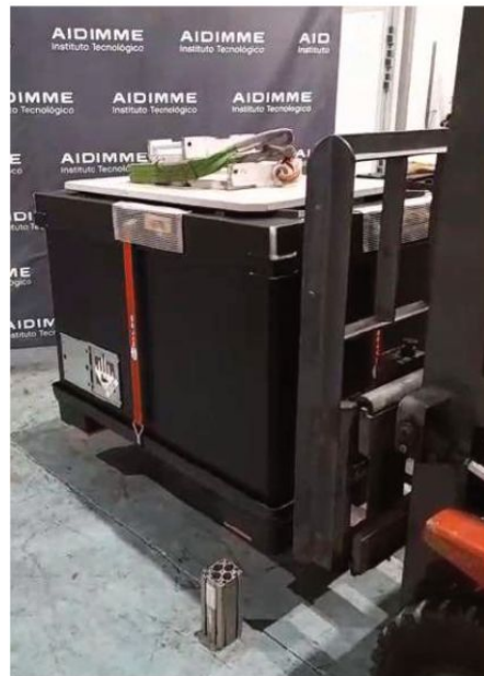
Photograph 2 - Bottom lift test in process
